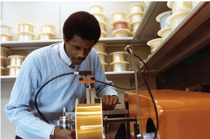
Alfred G. Richardson designs and produces samples of prototype lightwave undersea telephone cable in 1982. AT&T ARCHIVES AND HISTORY CENTER
