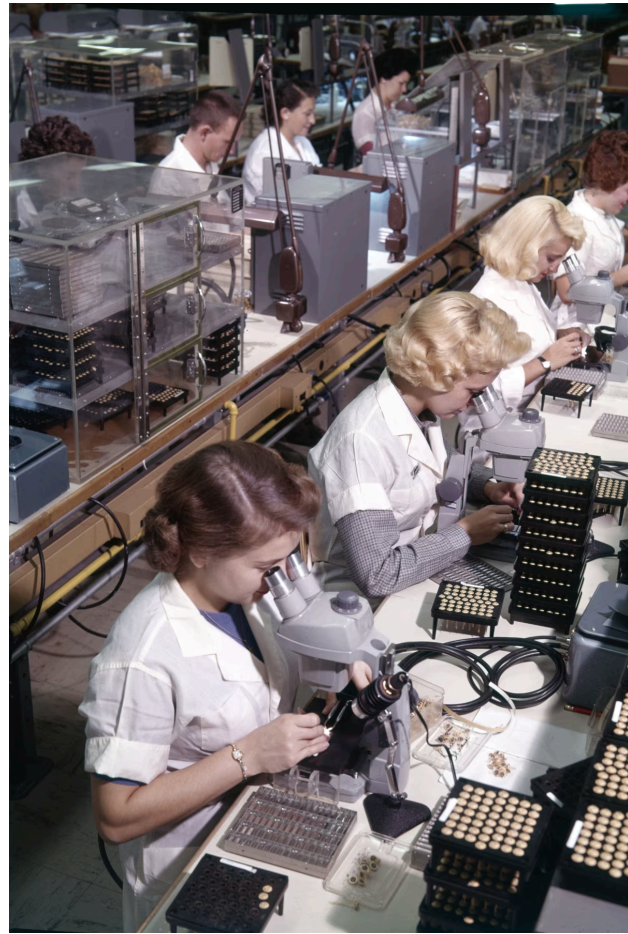
Inspecting a transistor (held with tweezers), and transistor assembly at Western Electric's Allentown, Pa., plant in 1960.
